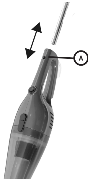
Fig 2. Inserting and releasing the handle Push the handle in until an audible 'click' is heard. Press button A to release handle.
